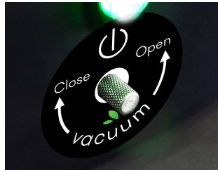
Turn the screw fully to the RIGHT to seal the chamber.
