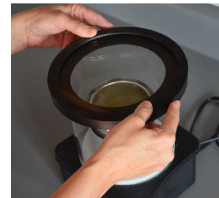
Place the lid on the collector.
