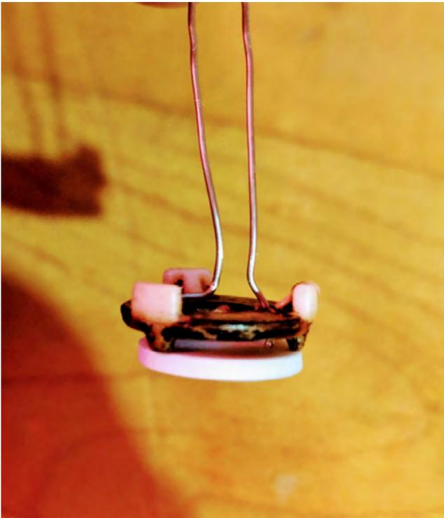
7: Put the assembled coil into the jig and bend on wire  $90^\circ$  towards the center then  $90^\circ$  straight up. The other lead is bent  $10^\circ$  towards the center then straight up.
